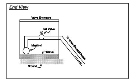
♦ The disposal trenches must be fed from the **top** of a manifold pipe.
