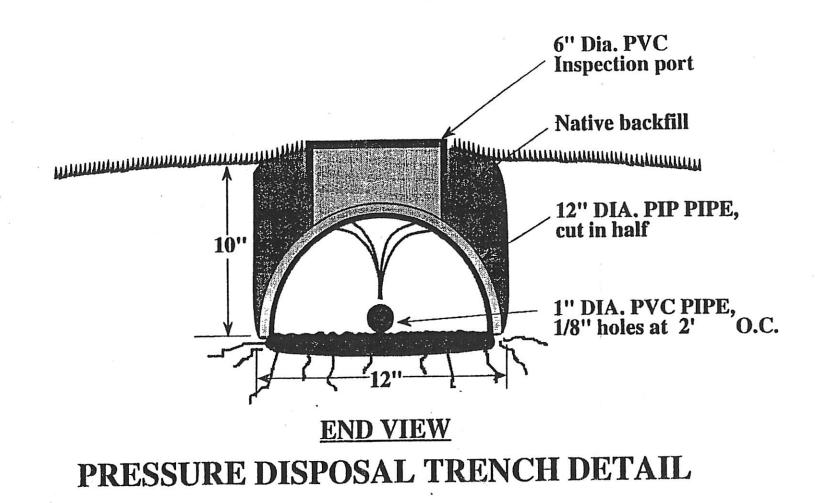
**Note:** If Infiltrator Chambers (Quick4 EQ24 LP) or EZ-Flow 1001P Bundles are to be used in lieu of the 12" plastic irrigation pipe for the gravelless absorption method, the products must be installed in accordance with the manufacturer's instructions.
