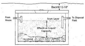
As the tank fills with sludge and grease, efficiency of treatment decreases. It must be periodically removed by pumping out the septic tank contents, which will be discussed in a later section.
